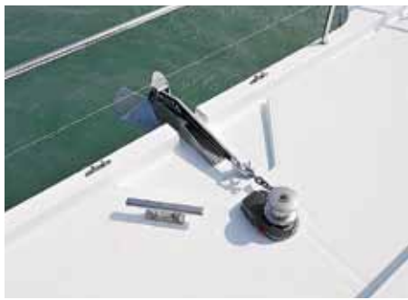
Very clear access to the bow roller and windlass, the chain feeds back to a locker just aft
