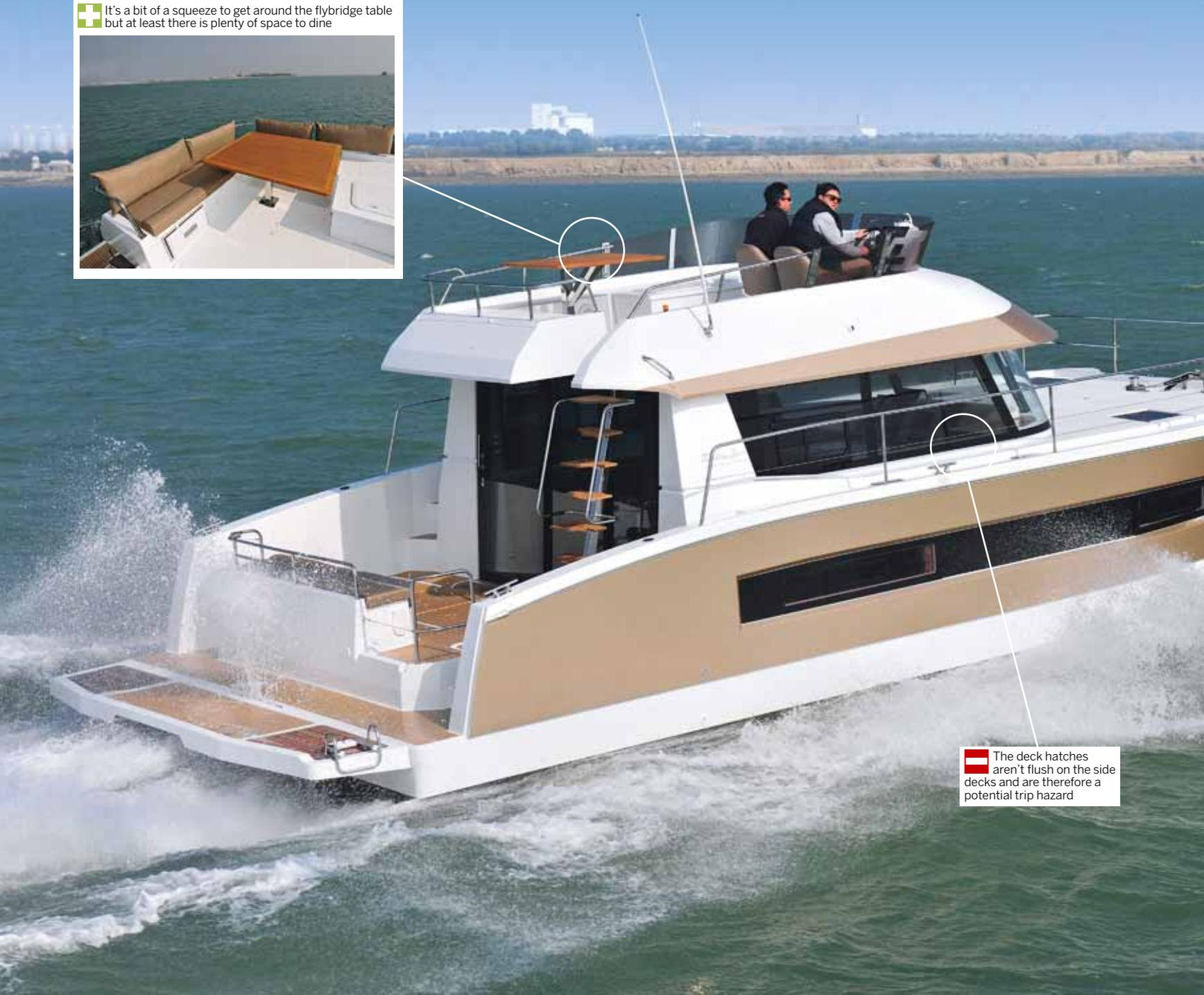
The deck hatches aren't flush on the side decks and are therefore a potential trip hazard
