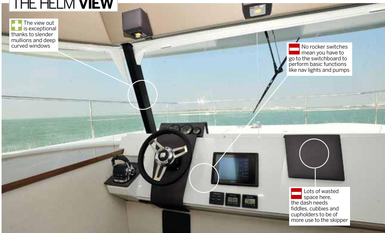
No rocker switches mean you have to go to the switchboard to perform basic functions like nav lights and pumps
