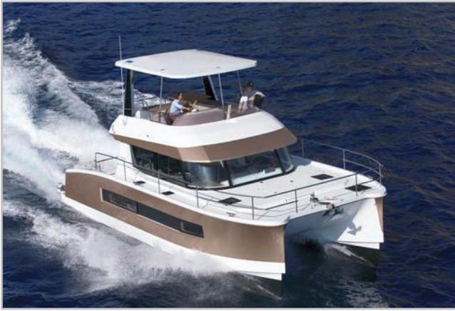
The hulls are fine at the waterline, but increase in volume above this with a marked step. This gives greater volume inside, and also deflects spray. ↑
